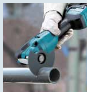
PVC pipe cutting
