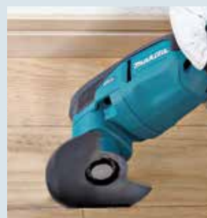
Cutout in the flooring
