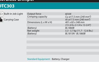
The weight may differ depending on the attachment (s), including the battery cartridge. The lightest and heaviest combinations are shown in the table.
