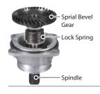
Lock Spring that joins Spindle and Sprial Bevel Gear protects the gears by absorbing shock casued accidental wheel lock during operation, ensuring longer tool life.
