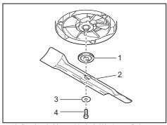
▶ 1. Bracket 2. Mower blade 3. Washer 4. Bolt
