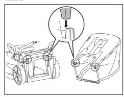
To remove the grass basket, perform the installation procedure in reverse.
