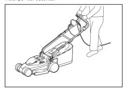
Start mowing near the power socket to ensure that the extension cord does not become an obstacle.
