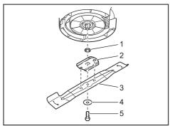
1. Spacer 2. Bracket 3. Mower blade 4. Washer 5. Bolt
