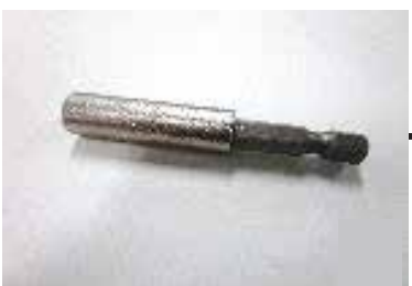
Magnetic bit holder (for power tool)
