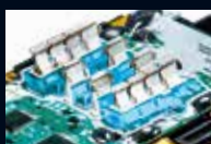
Terminal short-circuit prevention structure
