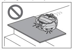
In such a place that the distance from a wall to a step is less than about 1 m, the robotic cleaner may fall while moving backward. Do not use the robotic cleaner where the distance from a wall to a step is less than about 1 m.
