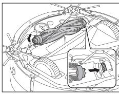
Rotate the bearing cap to align the orientation, then insert it into the robotic cleaner.
