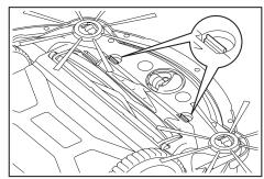
Remove the main brush cover.Do not disassemble the main brush cover.
