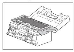
Close the filter-side top cover and make sure that the hook is hooked. Then, lock the two locking parts.
