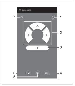
1. Power OFF button 2. Action buttons 3. Start/stop button 4. Sound ON/OFF button 5. Vacuum fan ON/OFF button 6. Location beacon buzzer/light button 7. Start point button
