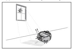
Do not use when there are objects such as carpets, mats, or plates near a step. If an object such as a carpet, mat, or plate is covering the step, the cliff sensor may not recognize the step correctly.
