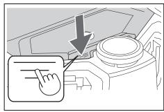
Remove the dust box.Do not hold the dust box with its opening facing downward. Doing so can cause dust to fall from the opening.
