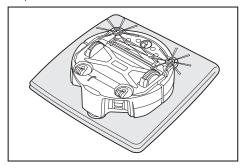
Do not press the undersurface of the robotic cleaner hard with the robotic cleaner turned upside down. Pressing it hard can cause damage to the robotic cleaner.
