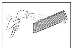
When the dirt of the dust box is noticeable, wash it with water or diluted neutral detergent.
