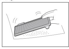
When the suction power of the robotic cleaner is weak, wash the filter with water
