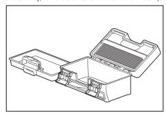
Put the dust case back in the dust box. Then, close the top cover and lock the two locking parts.
