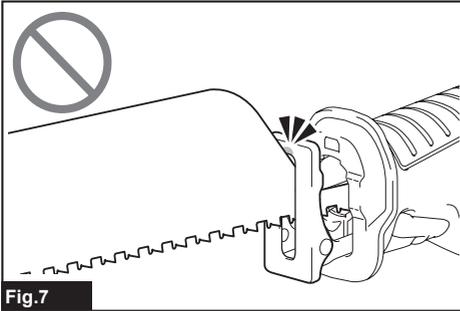
When the reciprocating saw blade loses its cutting efficiency in one place along its cutting edge, reposition the shoe to utilize a sharp, unused portion of its cutting edge. This will help to lengthen the life of the reciprocating saw blade.
