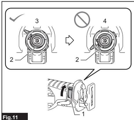
► 1. Release lever 2. Blade clamp sleeve 3. Released position 4. Fixed position
