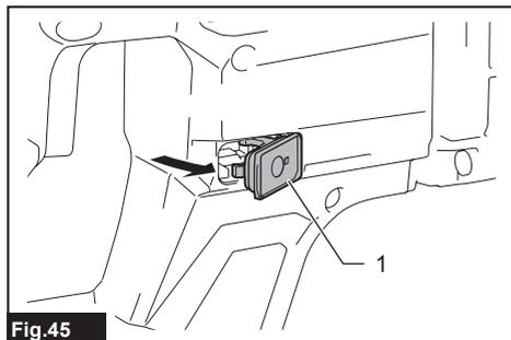
2. Insert the wireless unit to the slot and then close the lid.
