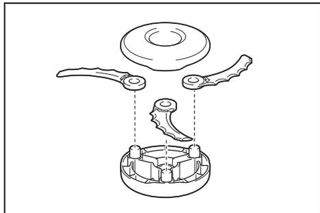
When installing the plastic blade, align the direction of the arrow on the blade with that of the protector.
