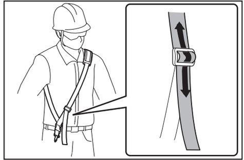
The shoulder harness features a means of quick release. Simply squeeze the sides of the buckle to release the tool from the shoulder harness.
