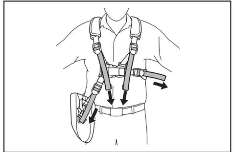
The shoulder harness features a means of quick release. Simply squeeze the sides of the buckle to release the shoulder harness.
