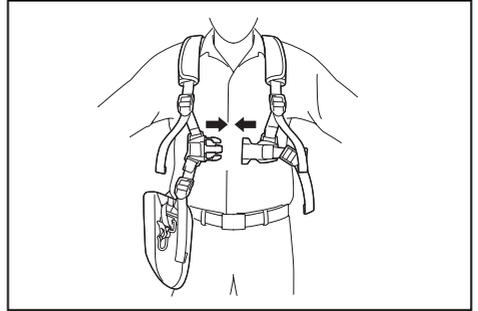
2. Clasp the hook on the shoulder harness to tool's hanger.
