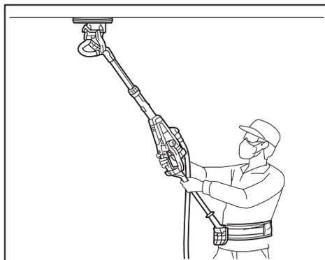
You can also operate the tool without using the belt and the holder as shown in the figure.
