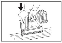
NOTE: If the head of the nail still remains above the workpiece even you hold the nail head, the material may not be suitable for the nailer. Continuing to use the nailer on such material may result in a damage to the driver of the nailer and/or nailer jamming.
