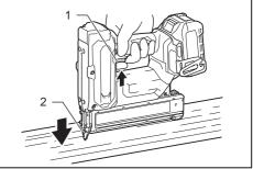
▶ 1. Switch trigger 2. Contact element
