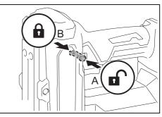
To prevent the switch trigger from accidentally pulled, the trigger-lock button is provided.
