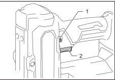
1. Trigger-lock button 2. Switch trigger
