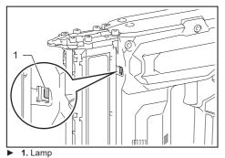
**NOTICE:** Use a dry cloth to wipe the dirt off the lens of the lamp. Be careful not to scratch the lens of lamp, or it may lower the illumination.
