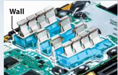
Terminal short-circuit prevention structure
