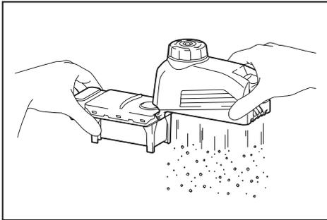
**NOTICE:** When cleaning the filter, tap the case of the filter gently by hand to remove dust. Do not tap the filter directly; touch the filter with brush or similar; or blow compressed air on the filter. Doing so may damage the filter.
