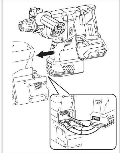
To remove the dust collection system, pull the tool while pressing the lock-off button.
