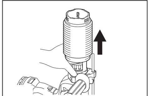
**NOTE:** If the cap comes off from the dust cup, attach it with its printed side facing up so that groove on the cap fits in the inside periphery of the attachment.
