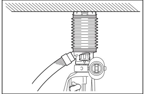
**NOTICE:** Do not use the dust cup set when drilling in metal or similar. It may damage the dust cup set due to the heat produced by small metal dust or similar.
