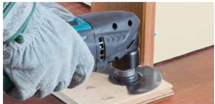
Wood flush cutting
