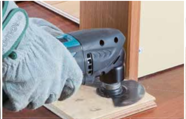
Wood flush cutting
