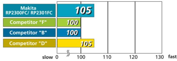
Bit used for tests: 12mm Cutting depth: 20mm
