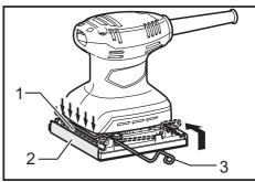
1. Clamping part 2. Abrasive paper 3. Lever
