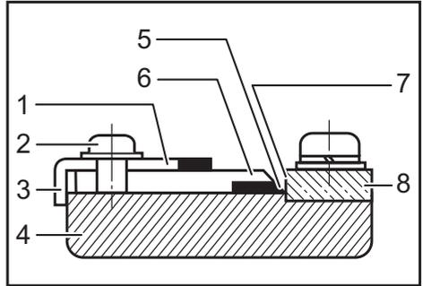
► 1. Adjust plate 2. Screws 3. Heel of adjust plate
