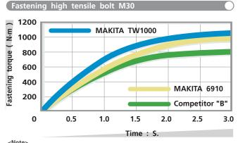
The definition of the max. fastening torque according to MAKITA standard; The figure which is measured at 3 seconds after start of driving, is the max. fastening torque in catalogue. The max. fastening torque of TW1000 is based on the same definition.
