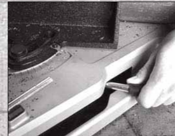
"Tool-less" guide plate adjustment for 0° - 45° miter cuts
