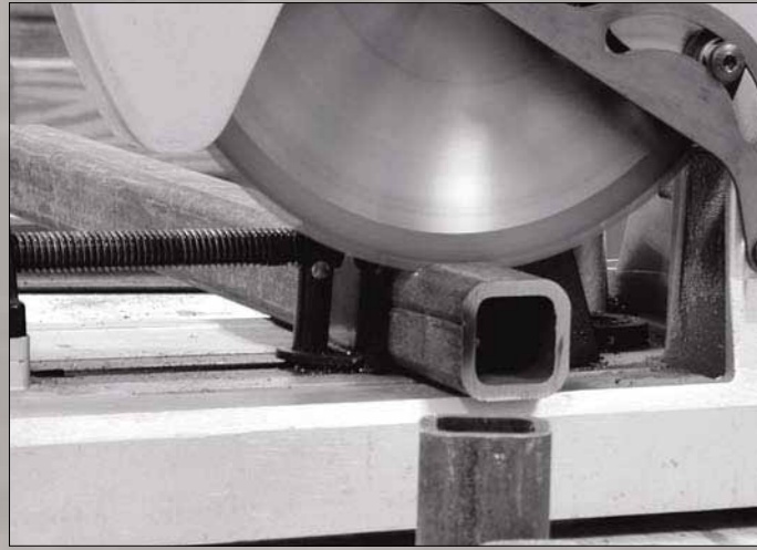
Carbide-Tipped Blades make Virtually Spark-Free Cuts
