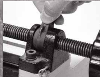
Quick release vise for fast repeat cut-offs
