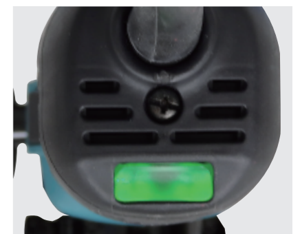
Even if plugged in with the switch "ON", the tool does not start with a blinking red light for visual warning.
