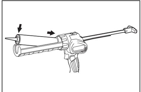
3. Push the rod gently until the piston touches the bottom of cartridge.
