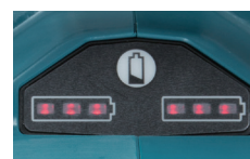
Battery capacity warning lamp
