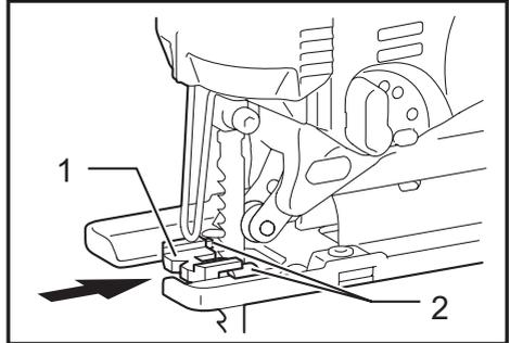
► 1. Anti-splintering device 2. Protrusions
