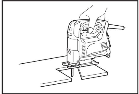
To trim edges or make dimensional adjustments, run the blade lightly along the cut edges.
